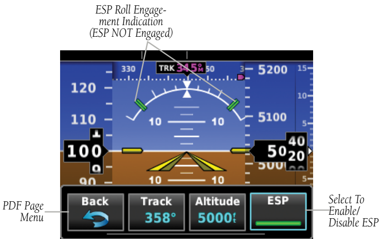
Figure 3-25 AFCS (ESP Enabled)
