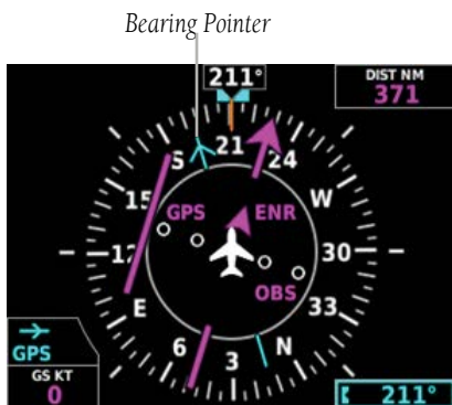
Figure 2-16 GPS Source Bearing Pointer
