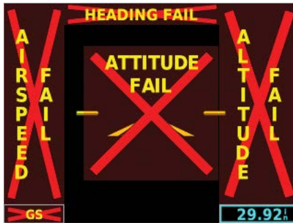
Figure 1-2 G5 PFD Page Failure Annunciations
