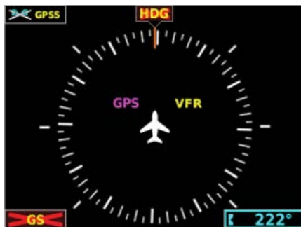
Figure 1-3 G5 HSI Page Failure Annunciations
