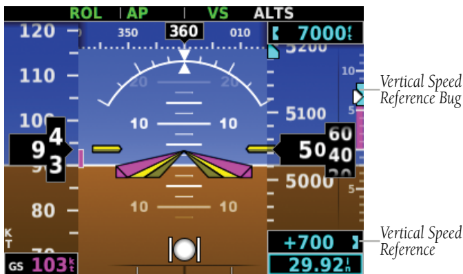
Figure 3-11 Vertical Speed Reference on PFD Page
