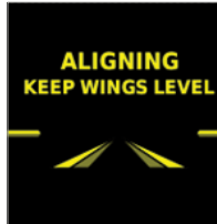
Figure 1-5 Attitude Aligned Keep Wings Level Indication
