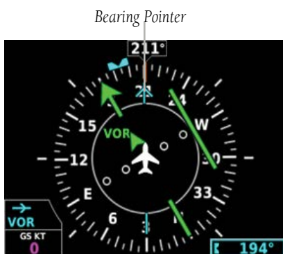
Figure 2-17 VOR Source Bearing Pointer
