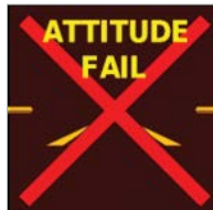
Figure 1-6 Attitude Failure Indication
