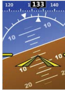
Figure 2-7 Ground Pointer Configuration
