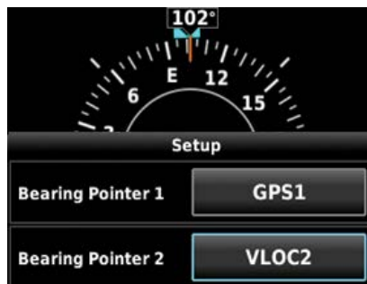
Figure 2-19 Bearing Pointer Setting
