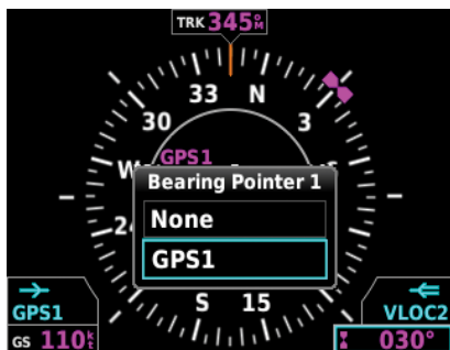
Figure 2-20 Bearing Pointer Source Options
