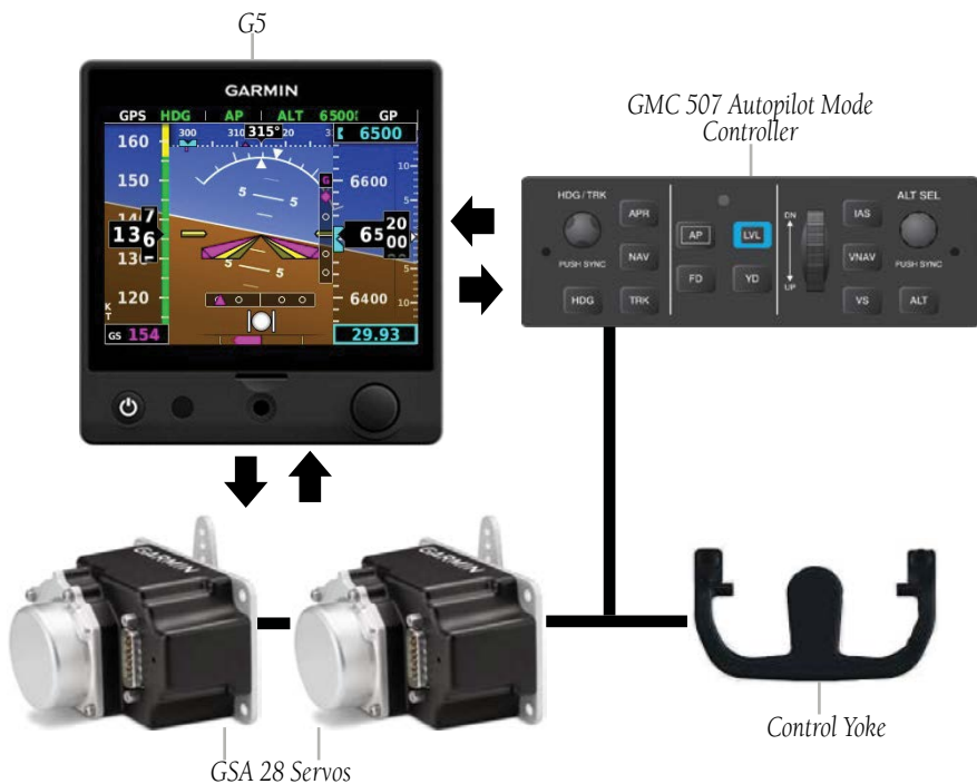
Figure 3-2 Core GFC 500 System
