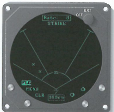
Figure 3-14. Weather View with a Heading Flag
