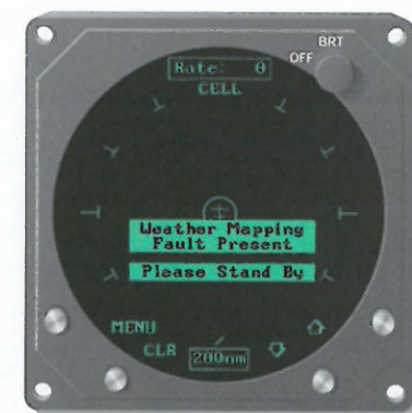
Figure 3-12. Weather Mapping Inhibited Screen
