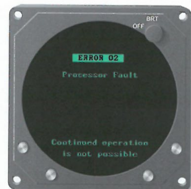
Figure 3-15. Error Message for a Fatal Fault
