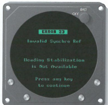
Figure 3-13. Error Message for a Heading-Related Fault
